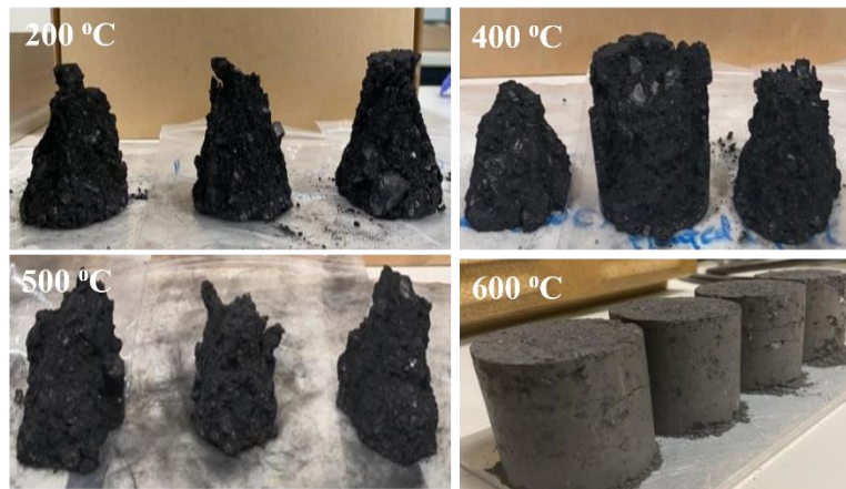
Figure 17. Form of failure for samples baked at different temperatures at 40 kN.
