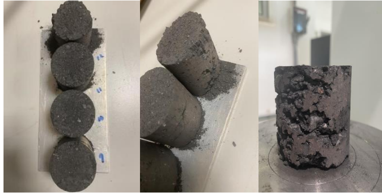
Figure 15. Before the compression test of 45 kN, Samples baked at 600 °C.
