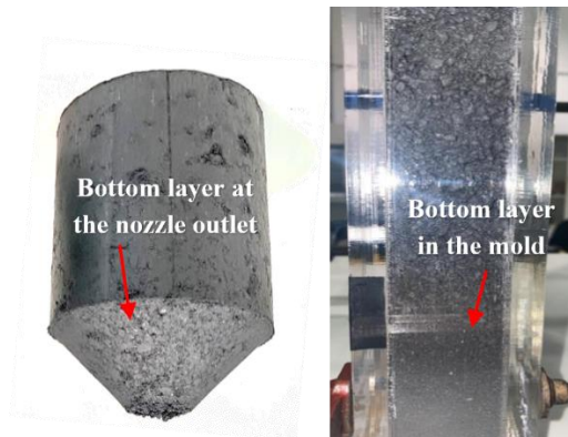
Figure 25. Compaction of paste comparison: injection through nozzle (left) and manual ramming (right).
