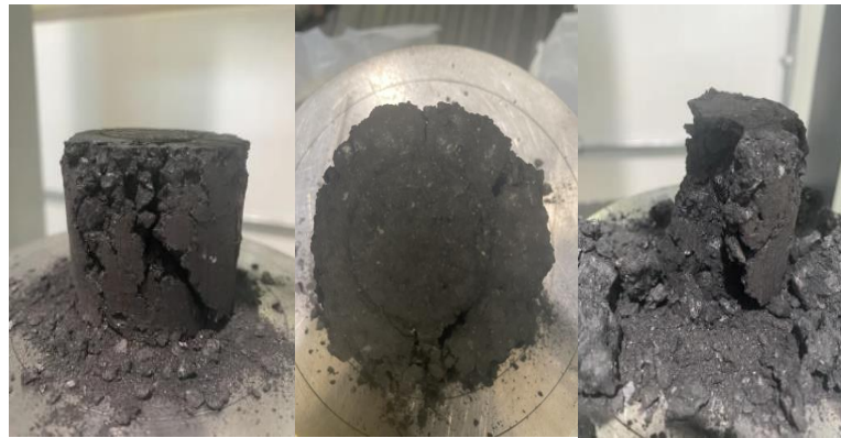
Figure 16. After the compression test of 45 kN, Samples baked at 600 °C.
