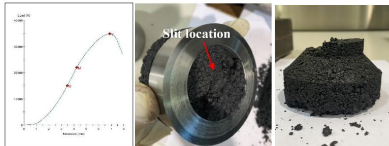
Figure 19. Graph from MTS machine showing load value of nearly 35 kN (left), no extrusion of the paste (middle and right).
