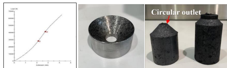
Figure 20. MTS showing load value up to 65 kN (left), with circular nozzle outlet (middle), similar results compared to first trial (right).
