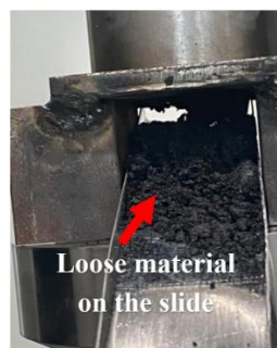
Figure 24. Ramming paste at the nozzle exit, sliding in the form of chunks.
